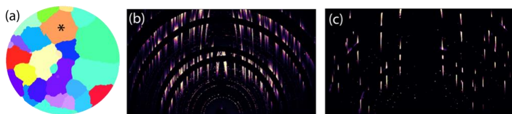
Figure 1: a) Grain map created using X-ray diffraction. b) Diffraction from polycrystalline Pd. c) Extracted diffraction from the grain marked with * in a.
